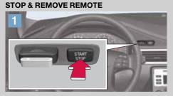
Park the car and push Start/Stop button to stop the engine.
